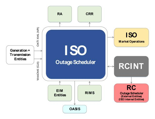
The OMS application is considered the primary interface for submission of outage information to the Long-Range, Short-Range, and Real Time outage processes that comprise the operations horizon, and serves as the conduit for the ISO CRR, RA, and RIMS processes.
